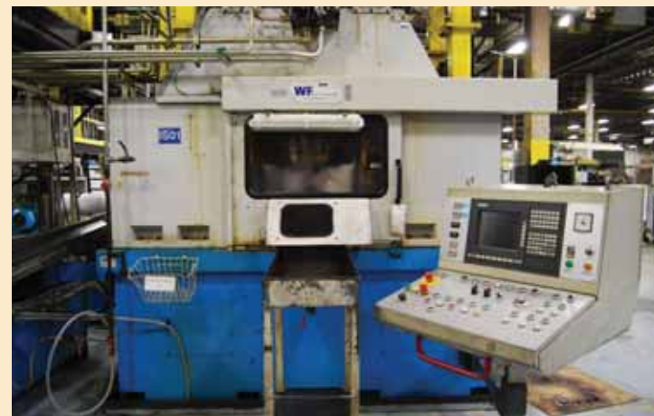
WF 'IVM 400' VERTICAL INTERNAL SPINNING MACHINE; S/N 10/7615 (2002), 11.4" Min. Workpiece Diameter, 13.78" Stroke of Ram Cylinder, 40 Ton Force of Ram Cylinder, 16 Ton Force of Eccentric Working Unit Radial Direction, 3.93" Stroke of Eccentric Working Unit Radial Direction, 5 Ton Force of Main Spindle Ejector, 3.93" Stroke of Main Spindle Ejector, 750 RPM Main Spindle, DIN 55027 Size 8 Main Spindle, Siemens 840C Control
