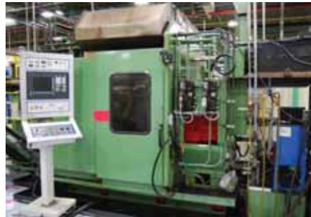
WF 'HBA 600S' HORIZONTAL HUB SPINNING MACHINE; (2004), Siemens Sinumerik Control
