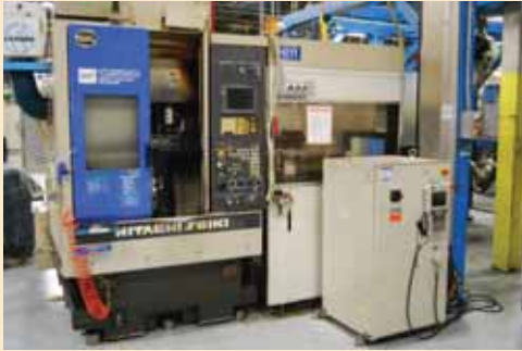
HITACHI-SEIKI 'CS20' INVERTED SPINDLE CNC LATHE; (Qty 3 – 1998/2000), 13.8" Max. Swing & Turning Diameter, 6" Max. Working Length, 51.57" X-Axis Travel, 14.57" Z-Axis Travel, 2.3" Spindle Bore, 30–5,000 RPM, Seicos 21L Control
