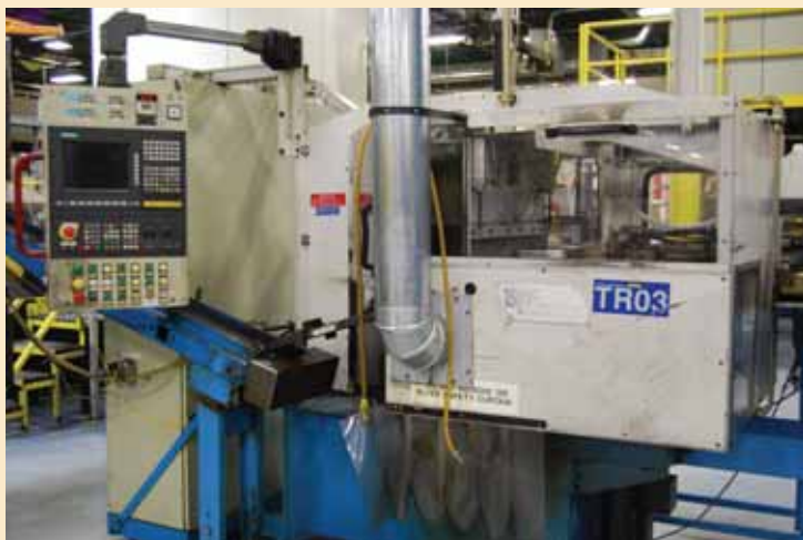
WF 'VAD 300' VERTICAL EDGE TRIMMING MACHINE; S/N 10/7799 & 10/7738 (Qty 2 – 2002), 3.54" Min.–9.84" Max. Workpiece Diameter, 0.157" Min.–2.95" Max. Workpiece Height, 7.87" Stroke of Slide in Vertical & Radial Direction, 3.93" Ejector Stroke, 2,000 RPM Main Spindle, DIN 55027 Size 6 Main Spindle, Siemens Sinumerik Control
