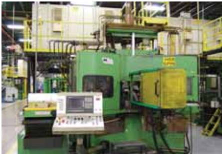
WF 'NAM 600' VERTICAL HUB SPINNING MACHINE; S/N 10/8992 (2004), 21.65" Max. Workpiece Diameter, 13.77" Stroke of Ram Cylinder, 30 Ton Max. Ram Cylinder Force, 16 Ton Max. Force of Spinning Slides in Vertical Direction, 16 Ton Max. Force of Spinning Slides in Horizontal Direction, 7.4" Stroke of Spinning Slides in Horizontal Direction, 5.9" Stroke of Spinning Slides in Vertical Direction, 5 Ton Max. Force of Main Spindle Ejector, 3.93" Stroke of Main Spindle Ejector, 0–750 RPM Main Spindle, Din 55027 Size 8 Main & Ram Spindle, Siemens Sinumerik 840 C Control
