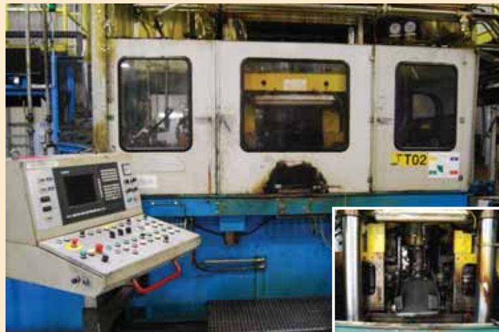
WF 'VB2BS' TWIN TURRET VERTICAL SPINNING MACHINE; S/N 10/6994 & 10/6976 (Qty 2 – 2000), 3.54" Min.–6.3" Max. Workpiece Diameter, 2.95" Max. Workpiece Height, 13.77" Stroke of Ram Cylinder, 60 Ton Force of Ram Cylinder, 20 Ton Force of Turret Head, (6) Rollers Per Turret Head, 7.08" Max. Roll Diameter, 5 Ton Force of Main Spindle & Ram Ejector, 750 RPM Main Spindle, DIN 55027 Size 8 Main Spindle, Siemens Control
