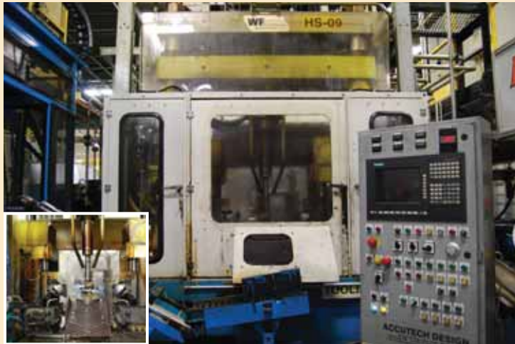
WF 'NAM 600' VERTICAL HUB SPINNING MACHINE; S/N 10/7198 (2002), 3.15" Min.–9.84" Max. Workpiece Diameter, 13.77" Stroke of Ram Cylinder, 30 Ton Max. Ram Cylinder Force, 15 Ton Max. Force of Spinning Slides in Vertical Direction, 15 Ton Max. Force of Spinning Slides in Horizontal Direction, 11.4" Stroke of Spinning Slides in Horizontal Direction, 5.9" Stroke of Spinning Slides in Vertical Direction, 5 Ton Max. Force of Main Spindle Ejector, 3.93" Stroke of Main Spindle Ejector, 250–600 RPM Main Spindle, Din 55027 Size 8 Main & Ram Spindle, Siemens Sinumerik 840 C Control
