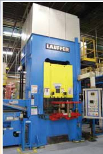
275 TON LAUFFER 'RA275' STRAIGHT SIDE HYDRAULIC PRESS; S/N 16705 (2002), 41" x 31.5" Bed Area, 42 Tons Retracting Pressure, 13.8" Ram Stroke, 24" Daylight, 260 Bar Max. Operating Pressure, PBK Automation Load/Unload, Siemens Simatic OP27 Control
