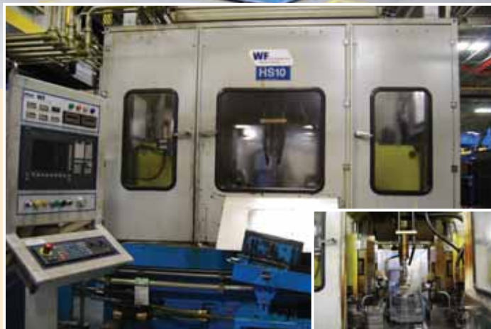
WF 'NAM 600' VERTICAL HUB SPINNING MACHINE; S/N 10/8992 (2004), 21.65" Max. Workpiece Diameter, 13.77" Stroke of Ram Cylinder, 30 Ton Max. Ram Cylinder Force, 16 Ton Max. Force of Spinning Slides in Vertical Direction, 16 Ton Max. Force of Spinning Slides in Horizontal Direction, 7.4" Stroke of Spinning Slides in Horizontal Direction, 5.9" Stroke of Spinning Slides in Vertical Direction, 5 Ton Max. Force of Main Spindle Ejector, 3.93" Stroke of Main Spindle Ejector, 0-750 RPM Main Spindle, Din 55027 Size 8 Main & Ram Spindle, Siemens Sinumerik 840 C Control
