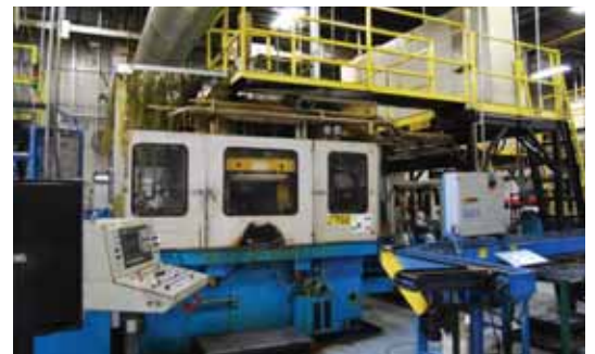
WF 'VB2BS' TWIN TURRET VERTICAL SPINNING MACHINE; S/N 10/6915, 10/6976 & 10/6994 (Qty 3 – 2000), 3.54" Min.–6.3" Max. Workpiece Diameter, 2.95" Max. Workpiece Height, 13.77" Stroke of Ram Cylinder, 60 Ton Force of Ram Cylinder, 20 Ton Force of Turret Head, (6) Rollers Per Turret Head, 7.08" Max. Roll Diameter, 5 Ton Force of Main Spindle & Ram Ejector, 750 RPM Main Spindle, DIN 55027 Size 8 Main Spindle, Siemens Control
